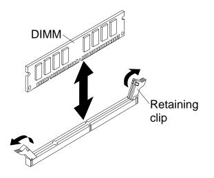
Note: DIMMs or DIMM fillers must occupy DIMM connectors 1, 2, 13, 14, 15, and 16 for proper cooling.
