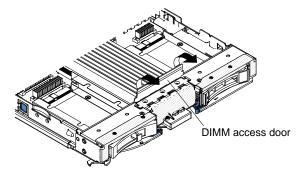
Step 10. Touch the static-protective package that contains the DIMM to any *unpainted* metal surface on the BladeCenter unit or any *unpainted* metal surface on any other grounded rack component in the
