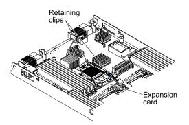
Step 7. Using your fingers, move the retaining clips away from the CIOv card; then, lift the card vertically out of the connector.
