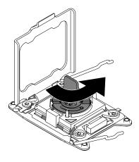
Figure 3. Installation tool handle adjustment
