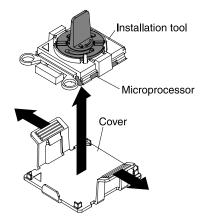
**Note:** Do not touch the microprocessor contacts. Contaminants on the microprocessor contacts, such as oil from your skin, can cause connection failures between the contacts and the socket.
