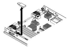
To install a USB module, complete the following steps:
