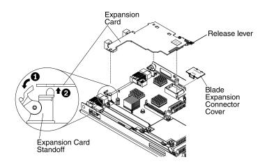
To remove a CFFh expansion card, complete the following steps:
