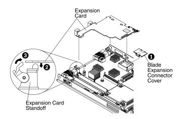
To install a CFFh expansion card, complete the following steps:
