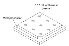
Step 5. Use the thermal-grease syringe to place nine uniformly spaced dots of 0.02 mL each on the top of the microprocessor.
