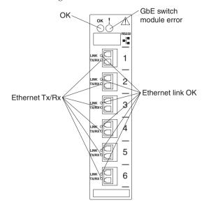
**Note:** An amber LED is lit when a system error or event has occurred. To identify the error or event, check the LEDs on the information panel of the GbE switch module. For additional information, see Chapter 6, "Solving problems," on page 33.
