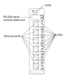
The following illustration shows the information panel for the fiber GbE switch module.
