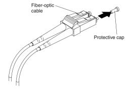
3. Connect the fiber-optic cable to the installed SFP module, as shown in the following illustration.
