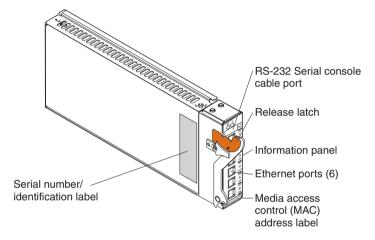
The following illustration shows the major components of the fiber GbE switch module.
