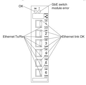
The following illustration shows the LEDs on the fiber GbE switch module.
