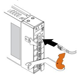
4. Check the LEDs on the switch module. When the switch module is operating correctly, the green link LED is lit. For information about the status of the switch module LEDs, see "LEDs" on page 29.
