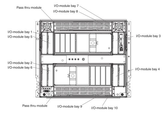
**Note:** An I/O module and expansion cards can also be installed in other I/O configurations. An expansion card that supports high-speed InfiniBand devices must be installed in each blade device that uses the I/O module. Expansion cards determine the BladeCenter unit I/O-module bays that
